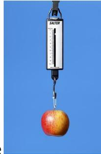
Newton meters are used to measure forces and can be used like
